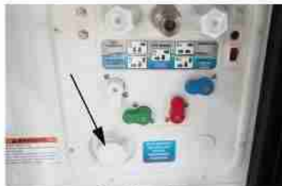
City Water Inlet (Located behind the drivers side service door) -Typical View
