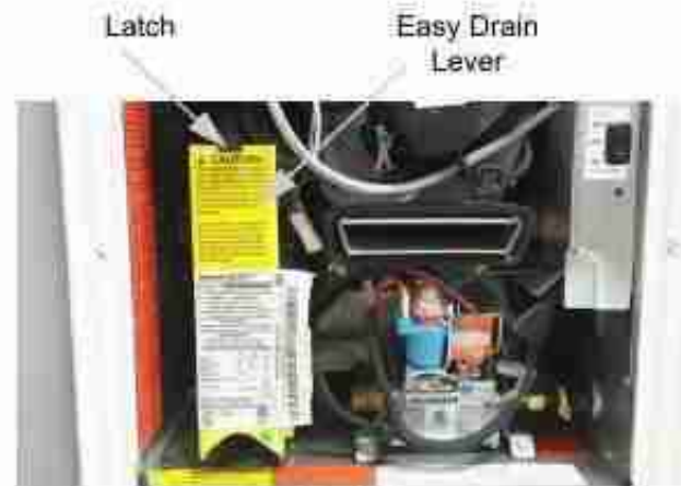
Easy Drain Lever (Located behind water heater access panel on exterior of the motorhome) -Typical View
