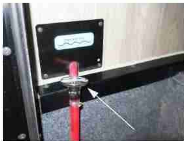
Tailgate Drain Valve (Model 622A) (Shown in the closed position) -Typical View
