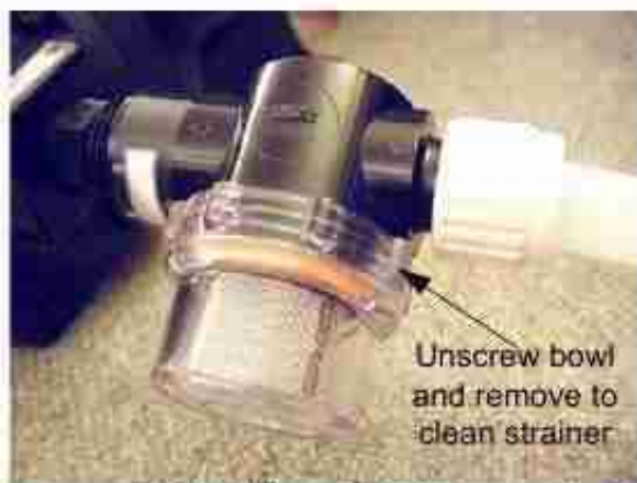
Water Pump Strainer -Typical View
