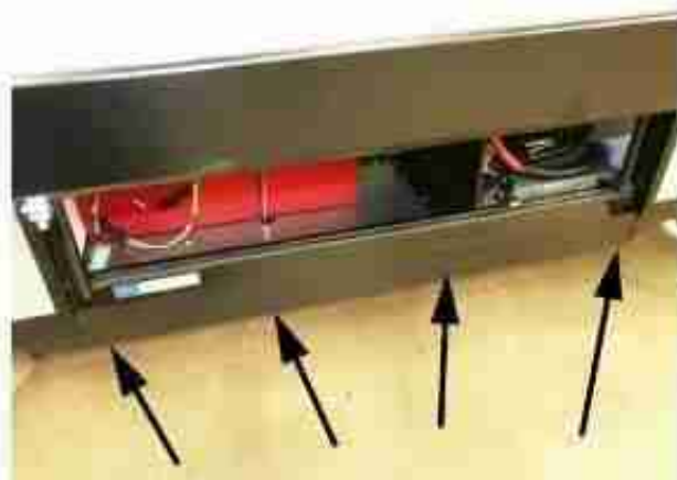
The 4 screws to remove the retention panel are located on the bottom. -Typical View
