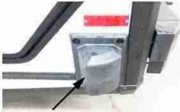
Driver side blind spot sensor location. Do not paint or cover this block. -Typical View
