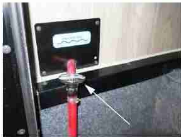
Drain the Tailgate Drain Valve (Shown in the closed position turn valve to open). (Model 622A) -Typical View
