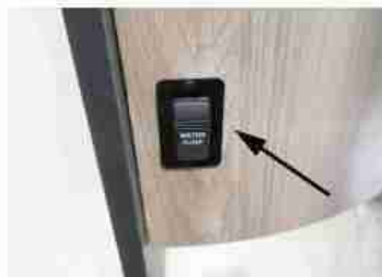
Water Pump Switch in the lavatory.
