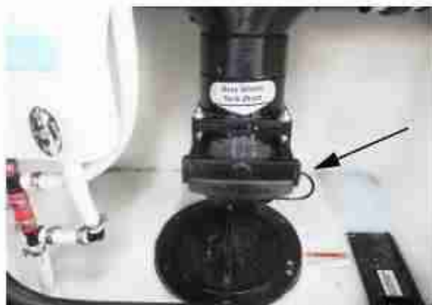
Sewage Drain Outlet with drain valve (Located inside the service center on the drivers side pull valve outward to open) - Model 622A shown
