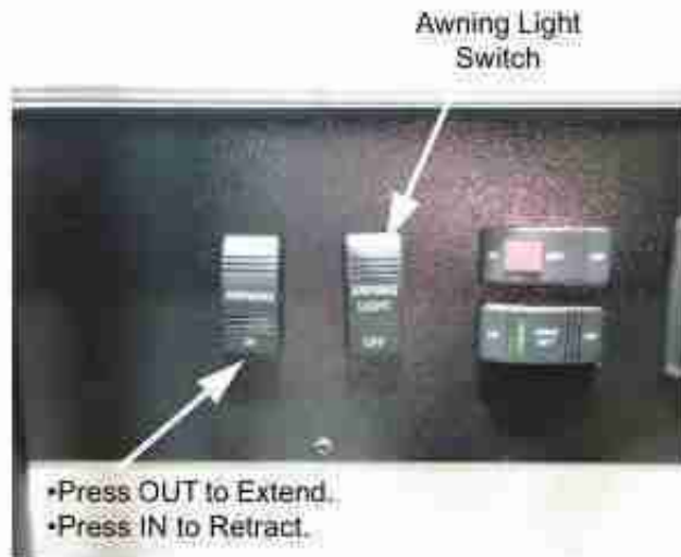
Power Awning and Awning Light Switches (Located near entrance door.) -Typical View
