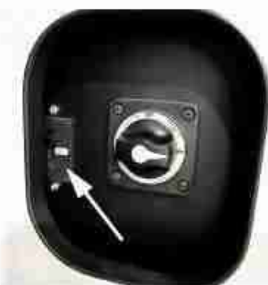
250 Amp circuit breaker (Located on the side of the dinette seat) -Typical View
