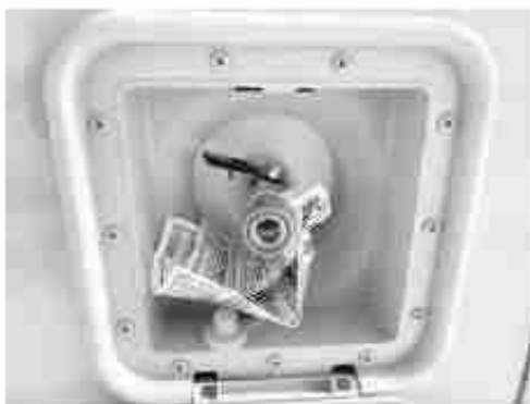
LP Quick Connect Port (shown open). Located on the passenger side. -Typical View
